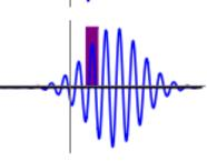
Propagation of a wave packet, with the motion of a single peak shaded in purple. The peaks move at the phase velocity while the overall packet moves at the group velocity.
